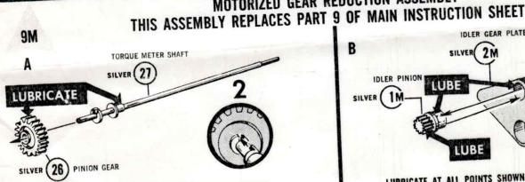
Cement 26 onto 27, locating-as shown in Small Drawing 2. Lubricate at all points shown and set aside to dry.
