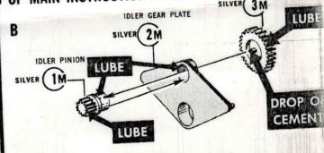
LUBRICATE AT ALL POINTS SHOWN Place, DO NOT CEMENT 1M into 2M. Place a drop of cement on pin 3M. Press pin on 3M into 1M.
